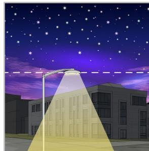
The Upward Light Ratio (ULR) and Upward Light Output Ratio (ULOR), the latter taking the flux from the luminaire into account, provide information on the percentage of light emitted towards the sky. This Schröder range of luminaires minimises or eliminates (depending on the options) upward-directed light flux. It complies with strict international and local requirements.
