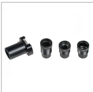
The GOBO version of the VALINTA series incorporates a standard SIZE E GOBO disc, ensuring compatibility and ease of use with an outer diameter (OD) of 37.5mm and an inside image (IA) of 28mm. Combined with a lens that offers three opening angles (17°, 25°, 30°), it allows for customised lighting effects. This adaptability makes it perfect for a variety of settings, from architectural features to event spaces and signage, providing precise illumination of the
